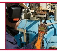
Rapidly detects benzene and total aromatic compounds (TACs) providing the most accurate, reliable data available.
