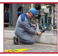
Designed for the search and location of flammable gases, GasCheck G rapidly detects the smallest of leaks.
