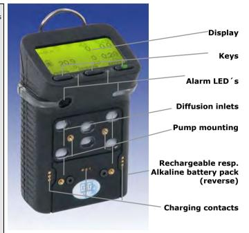
For a proper performance of the device it is necessary to notice, that all charging contacts will always kept clean. Dirt can be removed with a slightly wet piece of cloth. Do not use solvents or cleaning agents!
