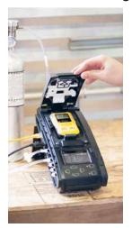
IntelliDoX combines smart-docking modules with our instrument management system to provide automated testing and record keeping for all Honeywell BW™ Clip4 detectors.
