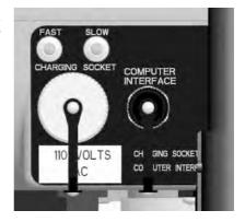
UNDER NO CIRCUMSTANCES MUST THE COVER BE REMOVED OR THE CHARGING LEAD BE CONNECTED TO THE UNIT WHEN IT IS LOCATED IN A HAZARDOUS AREA.
